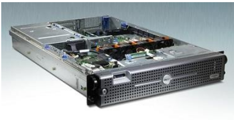
Server DELL PowerEdge 2950
